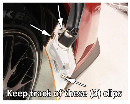
e. Behind each side marker is a single plastic fasten that needs to be removed. This fastener is a little tricky and may require a pick tool and or a bent awl.
