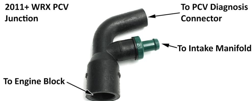
Picture above shows 2011+ WRX PCV Junction with PCV diagnosis connector removed from upper hose.
