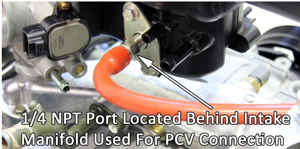
Above picture shows 2008-14 WRX manifold port for PCV connection.
