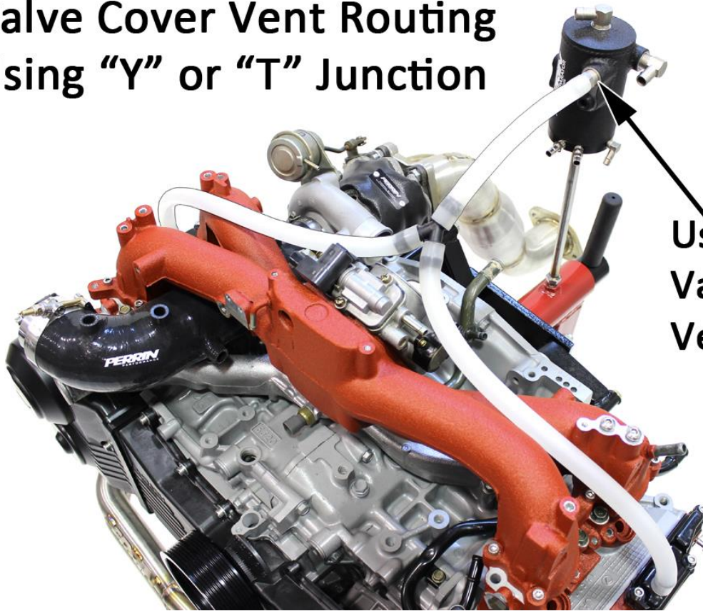
Diagram shows simplified hose routing for 2002-11 WRX and 2004+ STI model.
