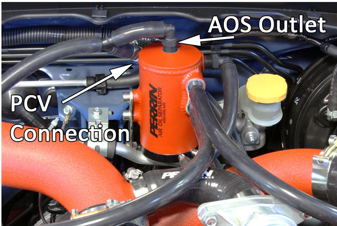
Above picture shows PCV connection on AOS outlet with hose routing behind AOS body.
