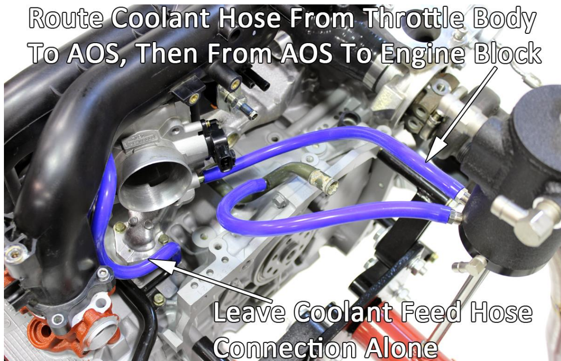
2008+ WRX coolant hose routing shown above. Diagram shows simplified path to help visualize routing.
