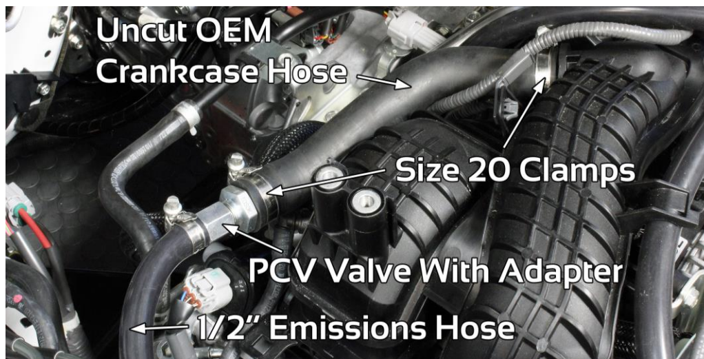
Above shows PCV hose rotated to right side of vehicle, then connecting to the AOS.
